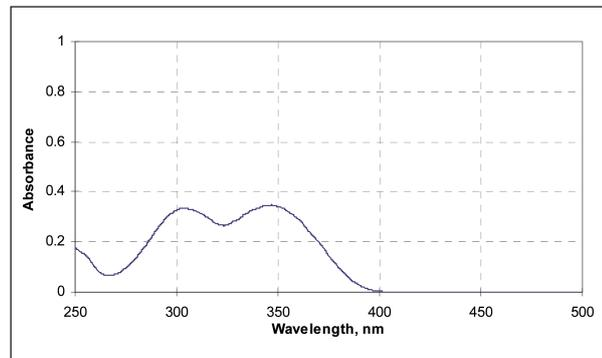
*Tinuin 234 exhibits high absorbance in the 300–400 nm region and minimal absorbance in the visible region (>400 nm) of the spectrum. The absorption maxima are at 302 nm and 343 nm ( $\epsilon = 16 \cdot 100 \text{ l/mol} \cdot \text{cm}$ ) in chloroform solution.*
